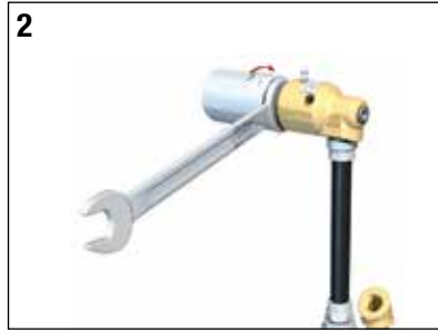
2 Install rotating union into machine.
